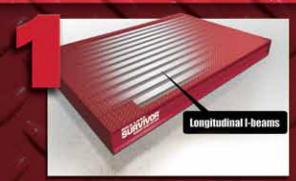
**Stronger Weighbridges:** Rice Lake truck scales typically have 25%-30% more structural steel content than competitive models. The SURVIVOR® OTR steel deck uses 5/16" checkered steel top plate, and (12) 12" wide flange 14 lbs per foot beams on 11-1/2" centers beneath the deck on the 11' wide model. The beams are welded to the top plate and the 3/4" end section weldment assemblies.
